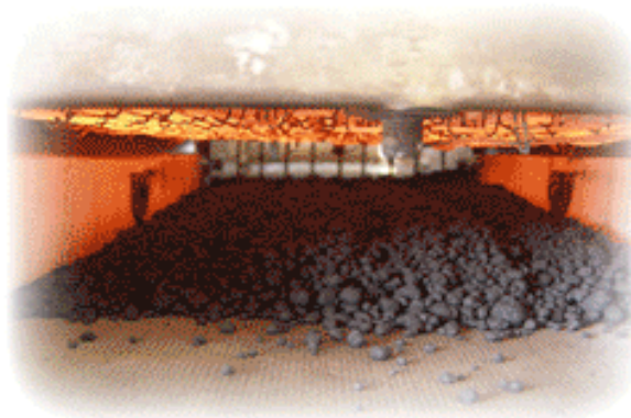
GRANULATED COAL DRYING 80% SOLIDS TO 90% SOLIDS EXTRUDED COAL DRYING 70% SOLIDS TO 90% SOLIDS
