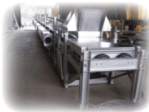
PNEUMATIC LINKED BELT TRACKING AND TENSIONING ENSURES PERFECT BELT ALIGNMENT
