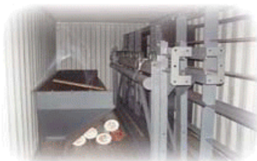
SCREENS OF 9 M 2 AND LARGER ARE BOLTED CONSTRUCTION AND CAN BE SEMI-ASSEMBLED FOR CONTAINERIZED TRANSPORT
